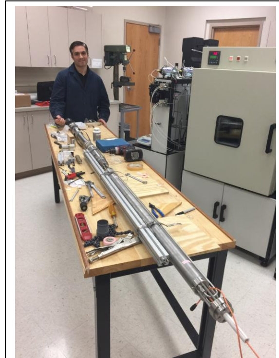
Figure 2. Photo of FluidTracer's borehole FluorFlow™ tool during assembly in EGI's lab. This portion of the tool shows only the spring-driven syringe pump and the tracer-ejection module. When completely assembled, the tool will measure approximately 18' in length and 2.875" in diameter.
